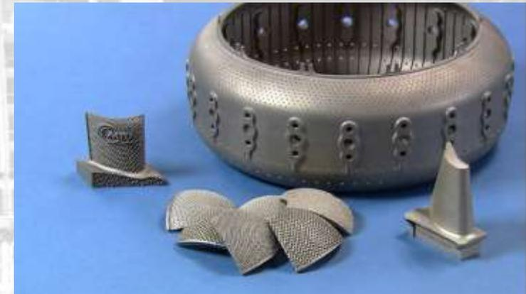
*3D printed parts by EOS for MTU Aero Engines*
